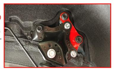
Using the jack, jack up the lower control arm on one side at a time to compress the suspension to ride height. This may take another jack or stand at the opposite front corner under the subframe to stop weight transfer.
